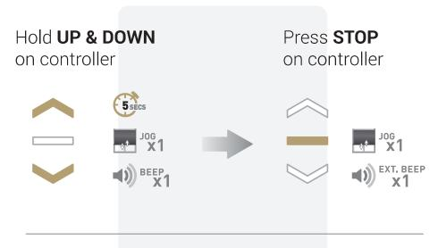
If motor is in Step Mode, use following steps to change to Roller Mode
