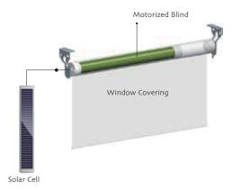
An extension cable can be offered if the distance between the motor shade and solar panel is far.
